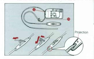
Attach the neckstrap to the neckstrap fixture (§) as illustrated. The projection on the neckstrap's rubber pad can be used to press the manual rewind button (§) or Quartz Date's setting adjustment button. You can also carry the camera by attaching the case to your belt as illustrated. You do not need to worry about forgetting or losing the case — just use the strap threading belt.
